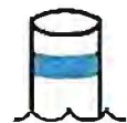
MOORING BUOY WHITE WITH BLUE BAND MAY SHOW WHITE REFLECTOR OR LIGHT
